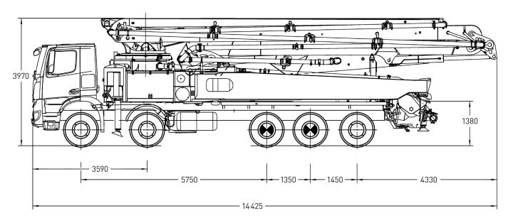
Note: Standard version. Dimensions and weights depend on truck, pump model and equipment. Dimensions in mm, MB-Arocs 4851, Euro 6. For illustration only.
