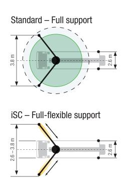
Dimensions can differ depending on configuration. Support width based on center of support leg.
