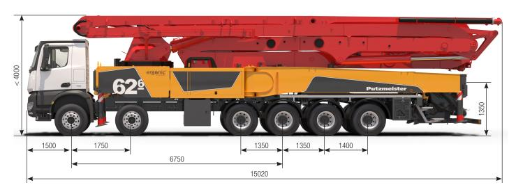
Note: Standard version. Dimensions and weights depend on truck, pump model and equipment. Dimensions in mm, MB-Arocs 6553 12x4 R6750 E6. For illustration only.
