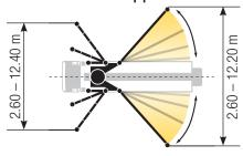
Dimensions can differ depending on configuration. Support width based on center of support leg.
