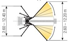
Dimensions can differ depending on configuration. Support width based on center of support leg.
