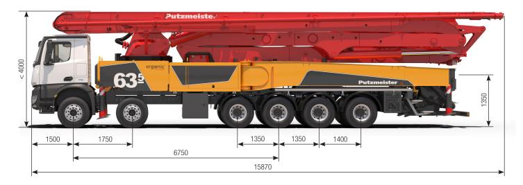
Note: Standard version. Dimensions and weights depend on truck, pump model and equipment. Dimensions in mm, MB-Arocs 6553 12x4 R6750 E6. For illustration only.
