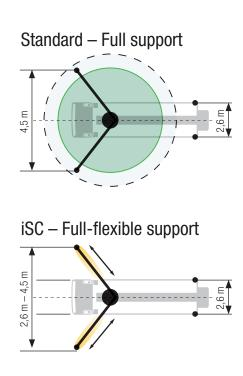
Dimensions can differ depending on configuration. Support width based on center of support leg.
