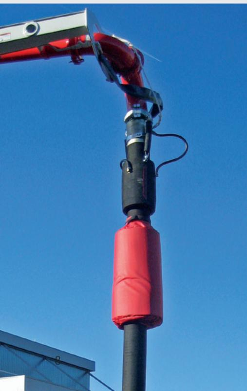
The central grease lubrication system on the boom reduces the time for daily maintenance
